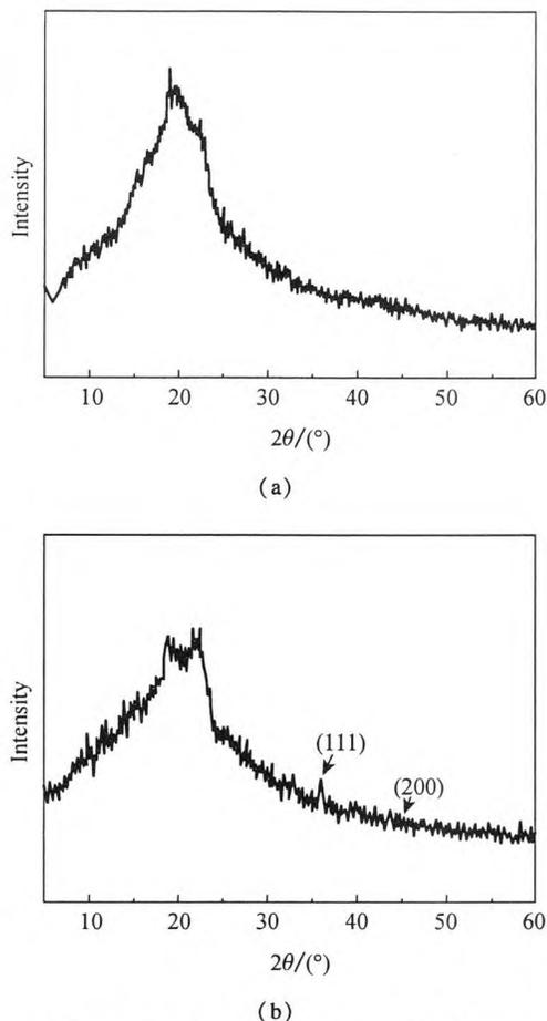
Fig. 8 XRD profiles of electrospun CS/PEO (80/20) nanofibers (a) without containing AgNPs and (b) containing AgNPs
