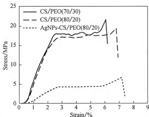
Fig. 9 Stress-strain curves of electrospun membranes with different CS/PEO ratios (70/30, 80/20, 80/20 with AgNPs)
