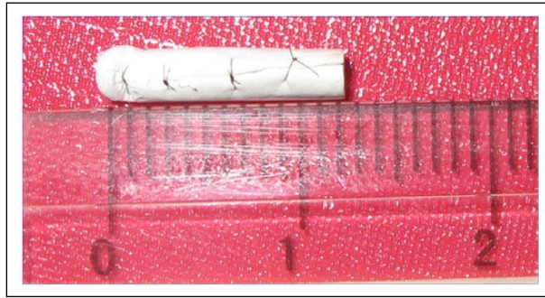
Figure 1. Exterior contour of the NGC (length = 12 mm, inner diameter = 1.4 mm, wall thickness = 0.3 mm).
