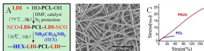
**Fig. 1.** (A) Synthesis route of the PEUU. (B) SEM of electrospun PEUU nanofibers. (C) Stress–strain curves of PEUU and PCL nanofibrous scaffolds.
