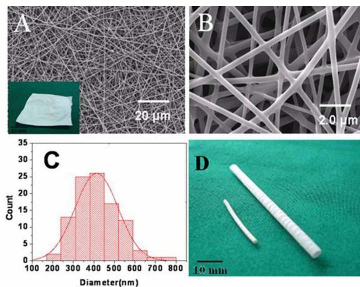
Figure 3. SEM micrographs (A, B), diameters distribution (C) and tubular fabrics (D) of core/shell nanofibers.
