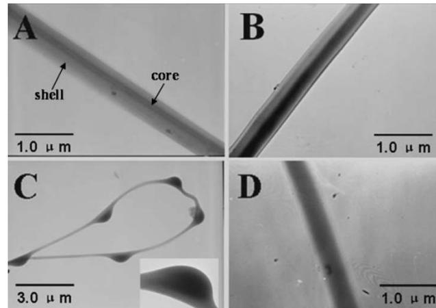
Figure 2. TEM micrographs of core/shell (A-C) and pure P(LLA-CL) (D) nanofibers. The proportions of feeding ratios between inner solution and outer solution were (A) 1:3, (B) 1:2 and (C) 1:1.
