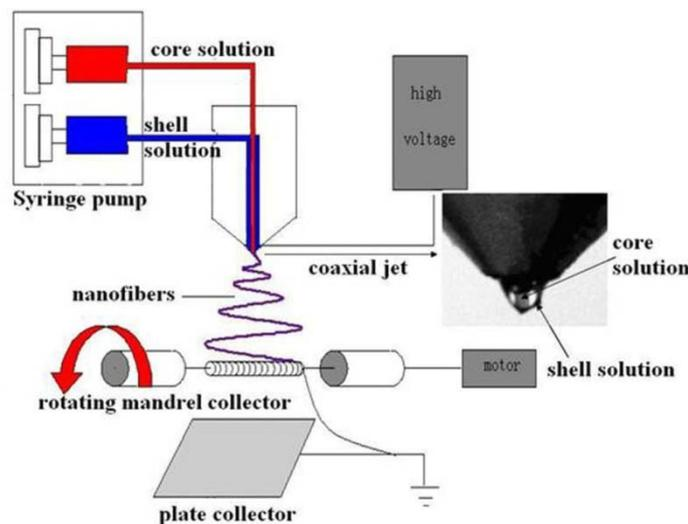
Figure 1. Illustration of fabricating core/shell nanofiber
